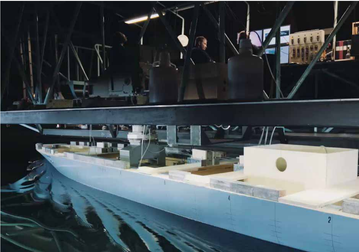
▲ Model tests of Wallenius Marine’s wind powered vessel concept at SSPA.
