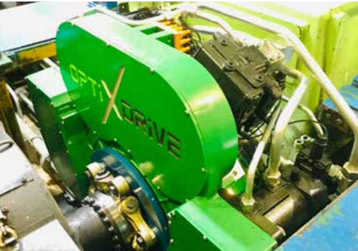
▲ Installed unit of the variable gearbox Optix-Drive.
