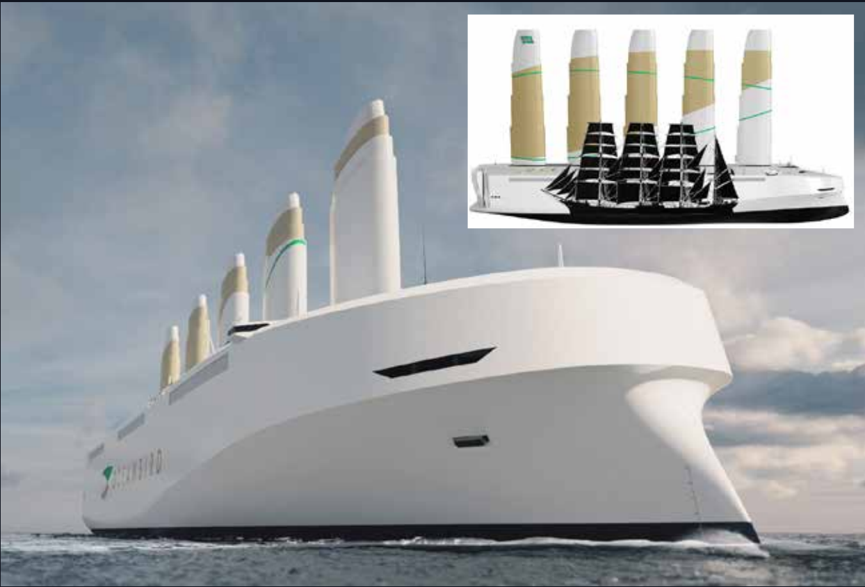
▲ Oceanbird with the telescopic wing sails in lowered position. Upper left: Sails fully erected, size comparison with the Pamir.
